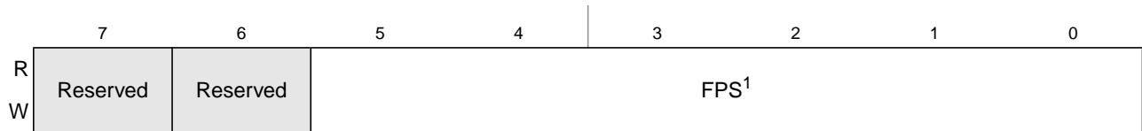
Figure 4-8. Flash Protection Register (FPROT)
