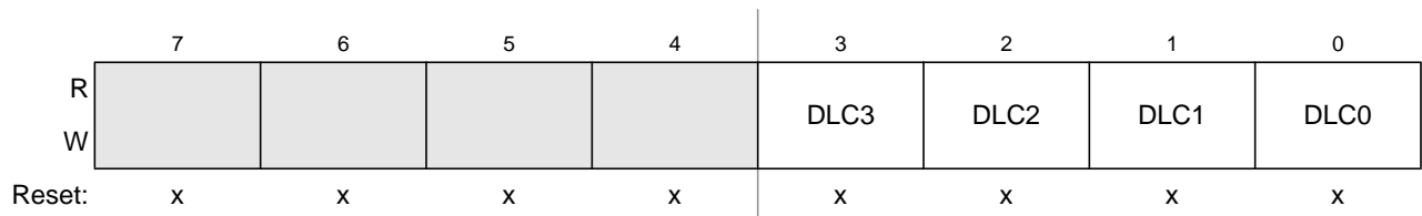
Figure 12-34. Data Length Register (DLR) — Extended Identifier Mapping
